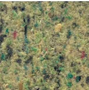
2,5 mm linoleum + 1,5 mm recycled foam
